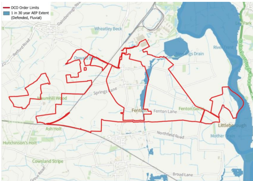
Figure 5.8: EA Flood Map for Planning, 1 in 30 year defended fluvial flood extent
